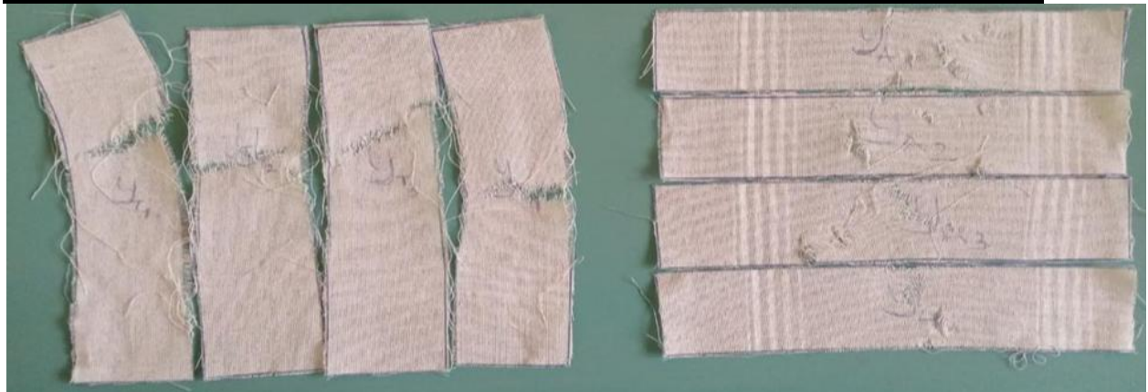
Figure 2. Condition of the fabric specimens after rupture. [4]
